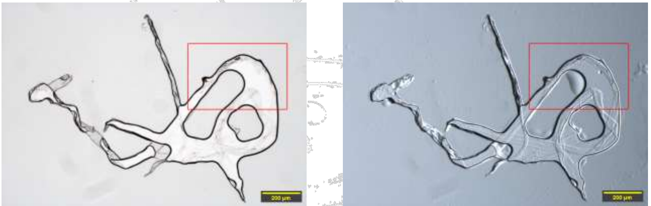
Image of a fabric fiber. Left: bright field. Right: oblique illumination.
